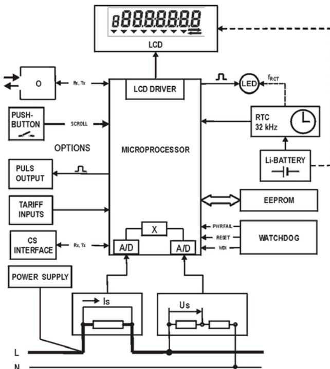
Fig. 6: Meter block-diagram
