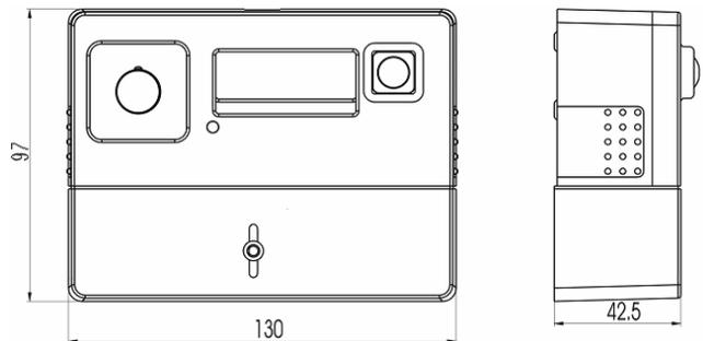
Fig. 5 – Meter with a short terminal cover
