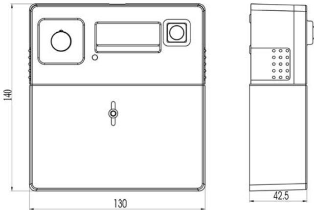
Fig. 4 – Meter with a long terminal cover
