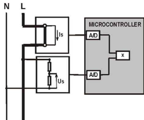
Fig. 7: Metering element
