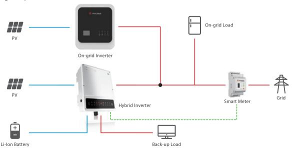
This solution integrates both hybrid and retrofit functions into a single system. In both on-grid systems as well as hybrids, the solar energy is used to supply electricity to both back-up loads and to charge the battery before the power is injected into the grid. By adopting such a solution, the system provides a more reliable source of supply for the loads, while ensuring a sufficient supply of green energy to charge the battery.
