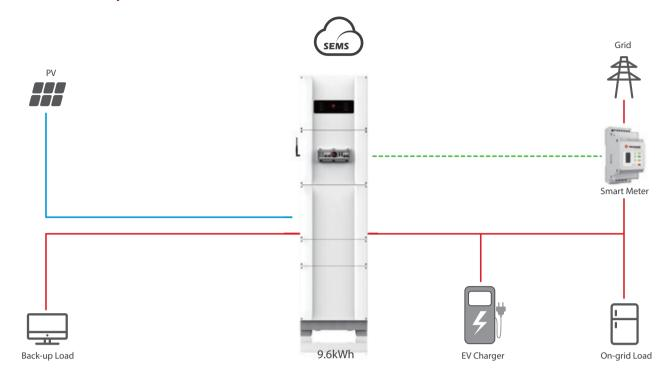
GoodWe is pleased to introduce the ESA Series, an "All-in-One" hybrid system that is designed to simplify the installation process to the maximum. It consists of the following elements: a hybrid inverter, a battery bank and a pre-wired system located inside a modern cabinet; it also includes connection devices and a preset cable slot. It is estimated that this system reduces the installation cost by as much as 60%!
