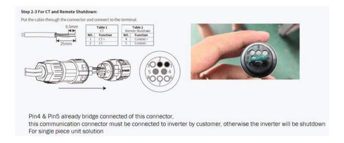
The example below shows the connector for the XS series inverters
